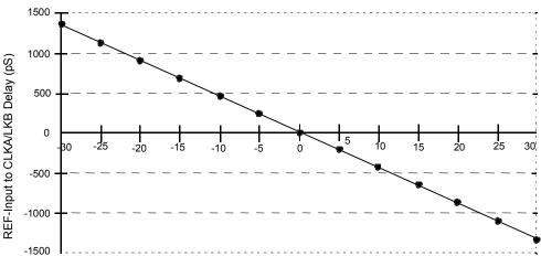
Output Load Difference: FBK Load - CLKA/CLKB Load (pF)
