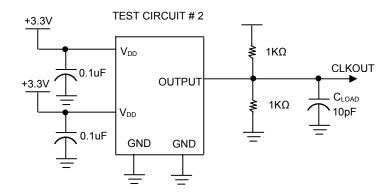
For parameter t<sub>8</sub> (output skew rate) on -1H devices
